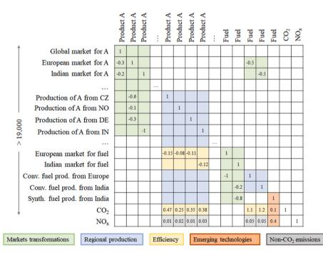
b) Simplified representation of transformations operated on the LCI database (positive values represent outputs, negative values represent inputs).
