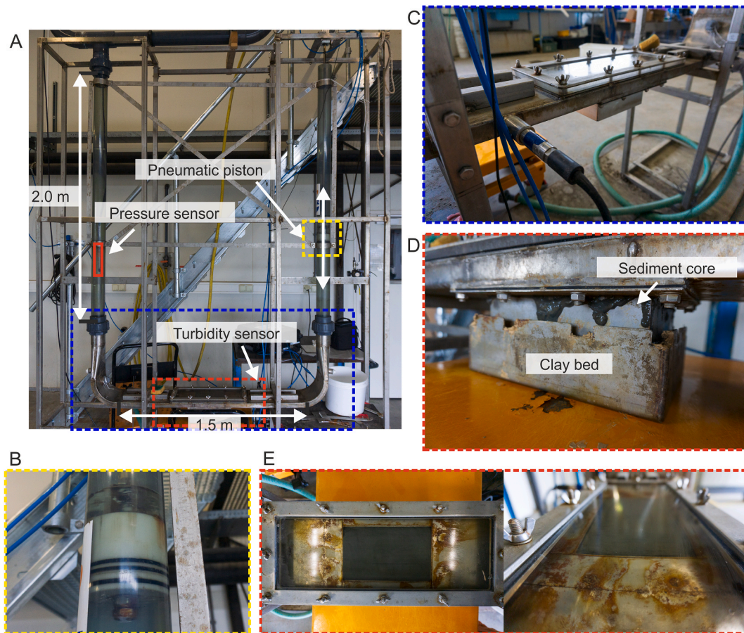
Fig. 1. The OsCaR-flume (A) is a U-tube type flume where a piston (B) forces oscillatory flow through a shallow channel (C). The flume and channel are secured by a metal frame to prevent vibrations from the movement of the piston. The sediment core is placed on top of a clay bed, which is used to make a watertight seal at the bottom of the sediment core (D). By pushing the sediment core into the clay bed the sediment can be raised out of the core and into the flume channel to ensure a smooth transition between the bottom of the flume channel and the sediment (E). Colored outlines in (A) correspond to outlines of closeups (B–E).
