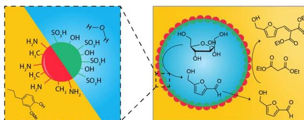
**Scheme 1.** Schematic representation of the use of bifunctional Janus A–B spheres for tandem PE catalysis. Left: Janus A–B particles get pinned at the oil/water interface, spatially localizing the two catalyst functionalities in the polar (acid) and nonpolar (base) phases. Right: The dehydration-Knoevenagel condensation reaction of fructose. Blue: water droplet; yellow: continuous organic phase.
