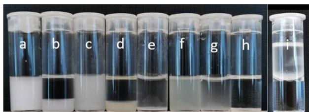
**Figure 3.** Unmodified  $\text{SiO}_2$  in water (a) and toluene (b);  $\text{SiO}_2\text{-NH}_2$  in water (c) and toluene (d);  $\text{SiO}_2\text{-NH}_2\text{-OSi}(\text{CH}_3)_3$  in water (e) and toluene (f); Janus A–B in water (g) and toluene (h). Amphiphilic Janus A–B particles quickly adsorbed at the water/toluene interface (i).
