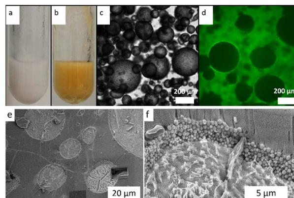
**Figure 4.** a, b) Physical appearance of the water/PG PE stabilized with 3.5 wt.% Janus A–B immediately after preparation (a) and after 24 h tandem catalysis (b). c) Optical microscopy image of the PE. d) Confocal fluorescence microscopy (CFM) image of the PE with the oil phase stained with Nile red. Scale bars of panels c and d = 200  $\mu\text{m}$ . e, f) Low- and high-magnification cryo-SEM image of water/PG PE stabilized with Janus A–B.
