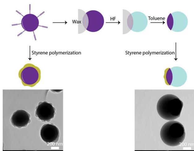
**Figure 2.** Schematic representation of styrene polymerization on vinyl-terminated  $\text{SiO}_2$  particles on homogeneous functionalized particles (left) and etched Janus particles (right) with corresponding TEM images after polymerization.
