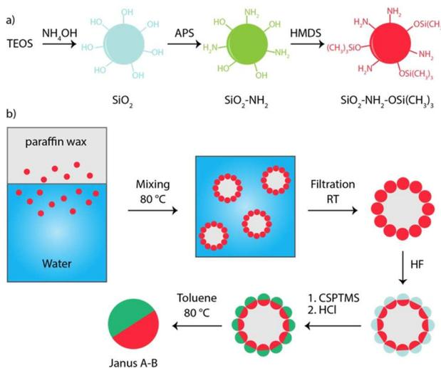
**Scheme 2.** a) Schematic representation of the synthesis of the monofunctional base-loaded and, hydrophobic particles synthesized from Stöber silica ( $\text{SiO}_2$ ). APS = (3-aminopropyl)triethoxysilane; HMDS = hexamethyldisilazane. b) Schematic representation of the synthesis of acid-base functionalized Janus particles using the solidified wax procedure. HF = hydrofluoric acid; CSPTMS = 2-(4-chlorosulfonylphenyl)ethyltrimethoxysilane.
