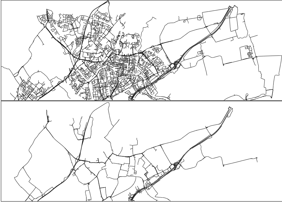
Figure 1.6: Top: Road network of the city of Leiden. Bottom: Heuristic generalization restricted to 30% of the total road length.
