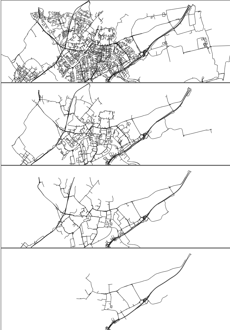
Figure 5.11: NSH under after application of the rescore heuristic with different budgets. The top image is the input graph, from the top down, the images correspond to a length budget of 50%, 30% and 10% of the input graph length, respectively.
