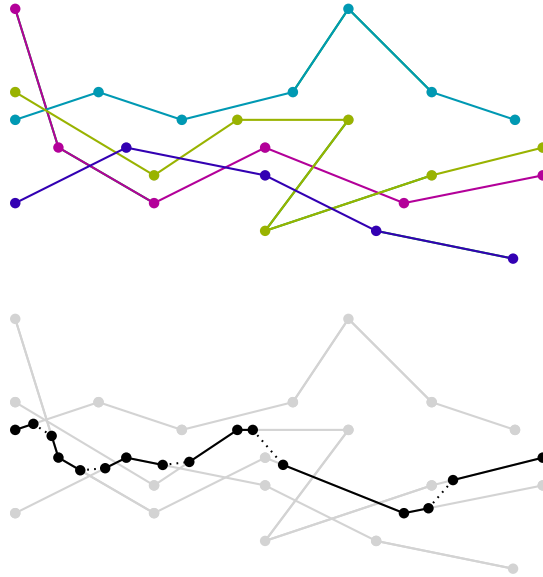
Figure 4.1: Top: A trajectory cluster where no trajectory is a good representative for the cluster. Bottom: A trajectoid constructed to be representative of the cluster. The dashed sections represent discontinuities where the trajectoid switches between trajectories. This can only occur when the points on both trajectories corresponding to the time of the switch are closer than the distance threshold \epsilon .
