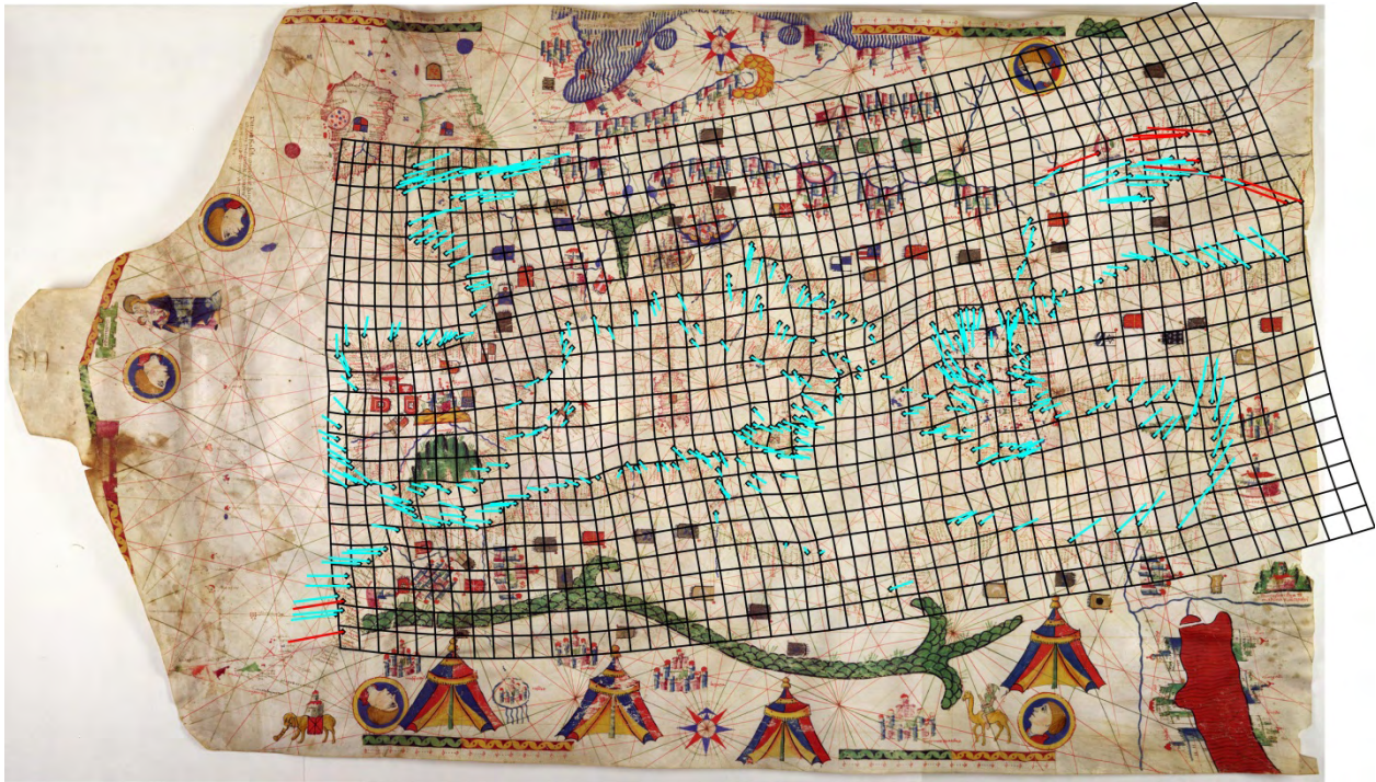
Figure 4: Portolan chart of Petrus Roselli (1466) with distortion grid and displacement vectors in 393 identical points shown as small blue squares. Points with residuals exceeding the threshold value are shown in red. (Portolan chart image by courtesy of the John Ford Bell Library, University of Minnesota).
