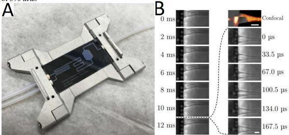
Figure 2: A) The glass/silicon Nanopede chip in the redesigned chip holder. Due to the removal of excess material on the side of the chip, high magnification lenses can reach the chip and image the nanoscale nozzles. B) The droplet production mechanism of the Nanopede. The left column shows the full formation cycle of one droplet, while the right column shows the moment of release at  $3x10^4$  frames per second. Images were procured using a full glass chip.
