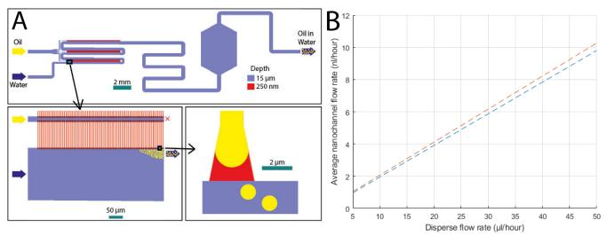
Figure 1:A) A schematic representation of the Nanopede chip. B) The spread of flow rates through single nanochannels for different incoming disperse flow rates. The dotted lines represent the maximum and minimum flow rates calculated.
