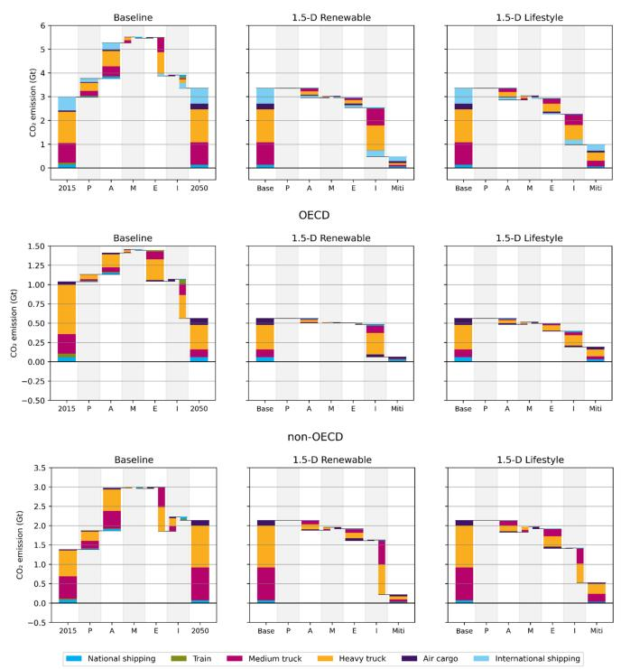
**Figure 8.** Changes in freight transport emissions between 2015 and 2050 (Baseline) and between the Baseline and mitigation scenarios (in 2050) due to different drivers. P: population; A: activity; M: mode, E: efficiency, I: carbon intensity (includes the impact of electrification). Emissions from international bunkers are only shown in global graph.
