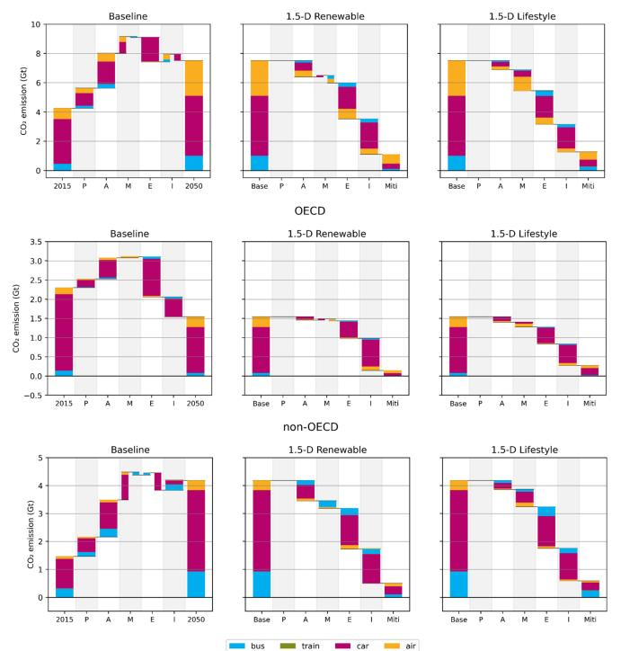
**Figure 6.** Changes in passenger travel emissions between 2015 and 2050 (Baseline) and between the Baseline and mitigation scenarios (in 2050) due to different drivers. P: population; A: activity; M: mode shift, E: efficiency, I: carbon intensity (includes the impact of electrification). Emissions from international bunkers are shown in global graph only.
