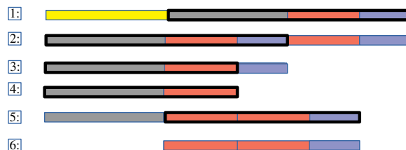
Figure 6. Macromutations to new behaviours: stages in the transition from the hand-designed seed replicator to the first self-scanning replicator. The black box outlines the part of the string that is written to the new mutant via the copy loop in the replication program. The colours indicate particular substrings (see text for details).
