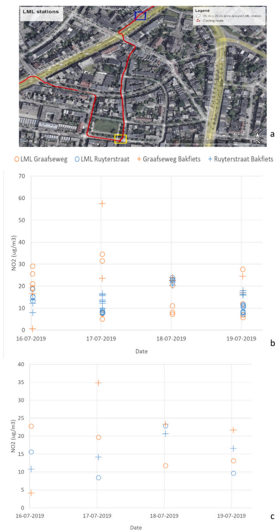
Fig. 3. Comparing the cargo-bike measurements with the Dutch national ground monitoring stations in the region. (a) Locations of the two ground stations, blue block is around the Graafseweg station and yellow the Ruyterstraat station. Bounding boxes (min latitude, max latitude, min longitude, max longitude) for the Graafseweg station are (51.84126, 51.84151, 5.85753, 5.85786) and for the Ruyterstraat station are (51.83810, 51.83830, 5.85701, 5.85719). The red line indicates the cargo-bike route. Within the two blocks the cargo-bike measurements are compared with the ground station measurements at the corresponding times. (b) The cargo-bike and ground station measurements while the cargo-bike was close to the ground stations. (c) Average values of the ground stations and the cargo-bike measurements.
