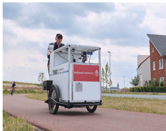
Fig. 1. The cargo-bike and instruments that are used to sensor the NO 2 in our study.
