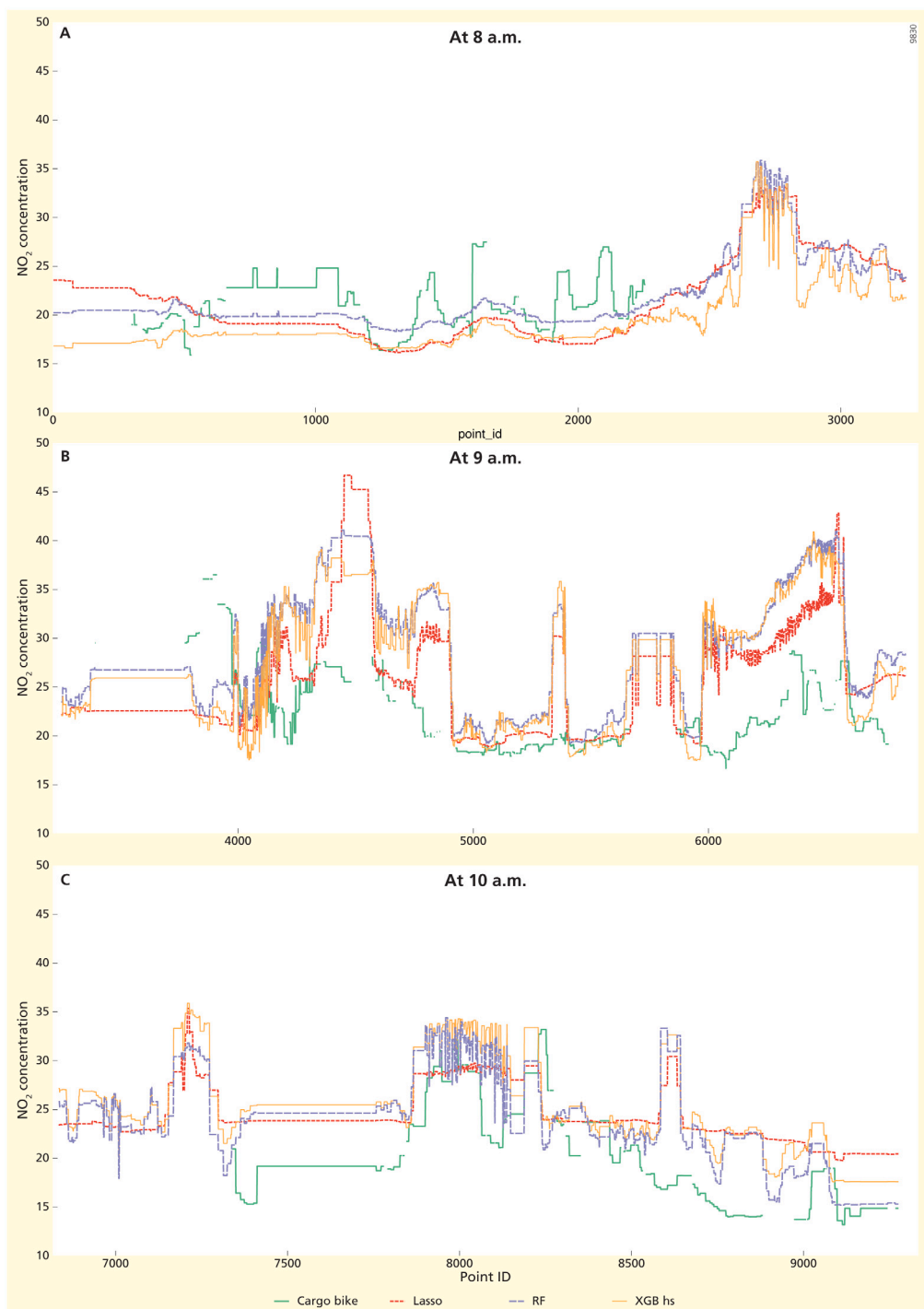
Fig. 6. Cargo-bike measurements and the XGB (high setting), RF, Lasso predictions and the cargo-bike measurements, visualised in the 1-D view. The point_id on the x-axis refers to the position on the track followed by the cargo bike.
