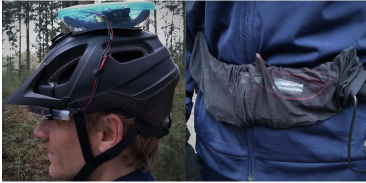
Fig. 5. The final feedback device prototypes used with the MTBalance system; the visual feedback device (top left) and the vibrotactile feedback device (top right).
