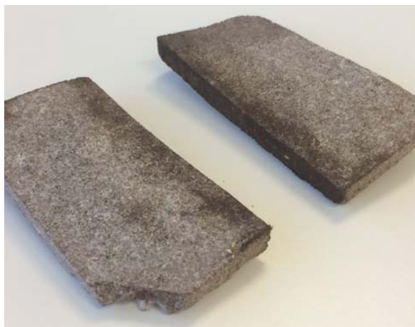
Fig. 7. Prototype of AF and SC composite after waterjet cutting
