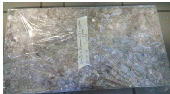
Fig. 3. Preparation of AF and SC composite in a mould
