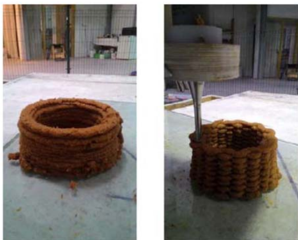
Fig. 9. 3D printing test and objects by Officina Corpuscoli, Co-de-iT and digifabTURING
