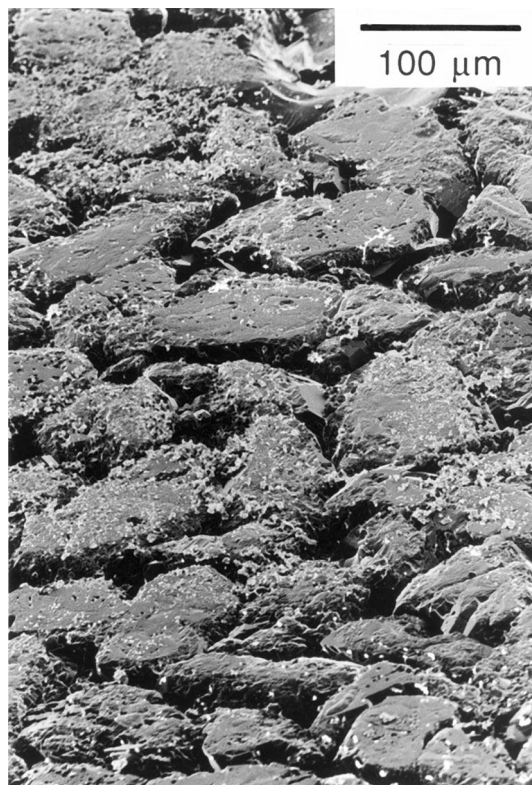
Figure 3. SEM micrograph showing top surface of the truncated quartz crystals after removal of the polished quartz plate. Note flat top surface of the grains.
