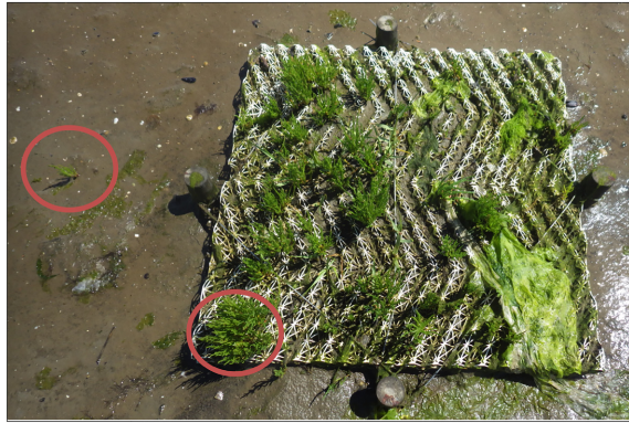
FIG. 5. Photograph of the artificial structure used in the field experiment on Texel, the Netherlands. The structure shown here has developed a raised internal sediment platform that supports high densities of salt-marsh recruits, predominantly Salicornia spp. Recruits found within the structure are also considerably larger than those found in the nearby unmodified mudflat (see individual comparison highlighting by the two red circles). Photo by Greg Fivash.
