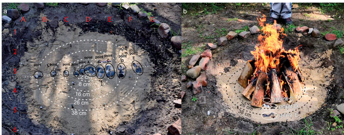
Fig. 6. Layout of fire 6 and 7 with indication of reference points and distance from the middle. a) Position of experimental tools and geological samples before the fire was built. b) Position of experimental tools visible for the heat camera during burning.
