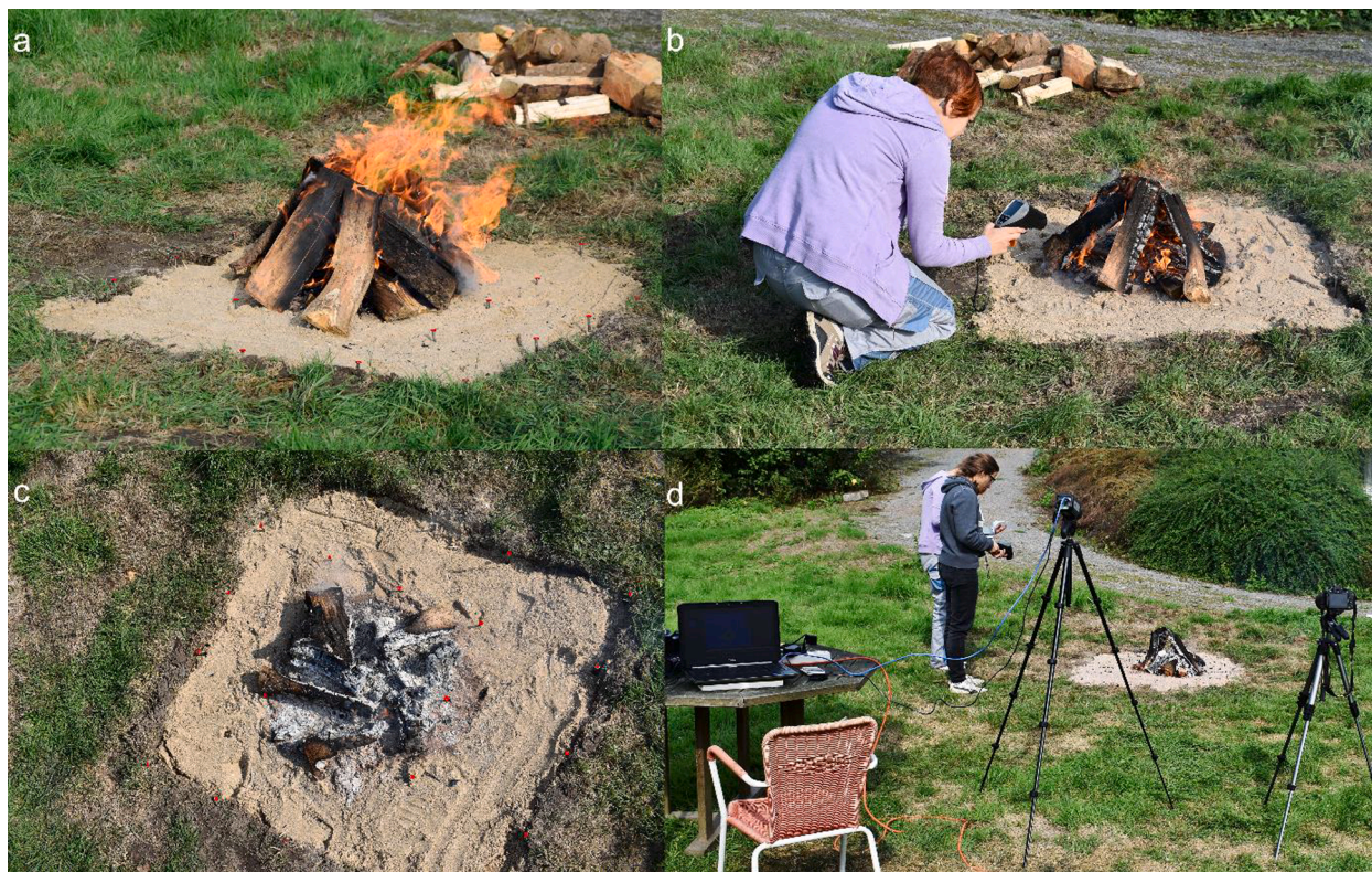
Fig. 2. Setting of fires without stone samples (fire 1–4) with equipment used for documentation. a) 1x1m square filled with river sand with fire made of pine wood. b) Measuring during fire with a Testo 835-T2 infrared thermometer. c) Top view of fire during smouldering. d) Setup of the FLIR A655sc heat camera and a DSLR camera.
