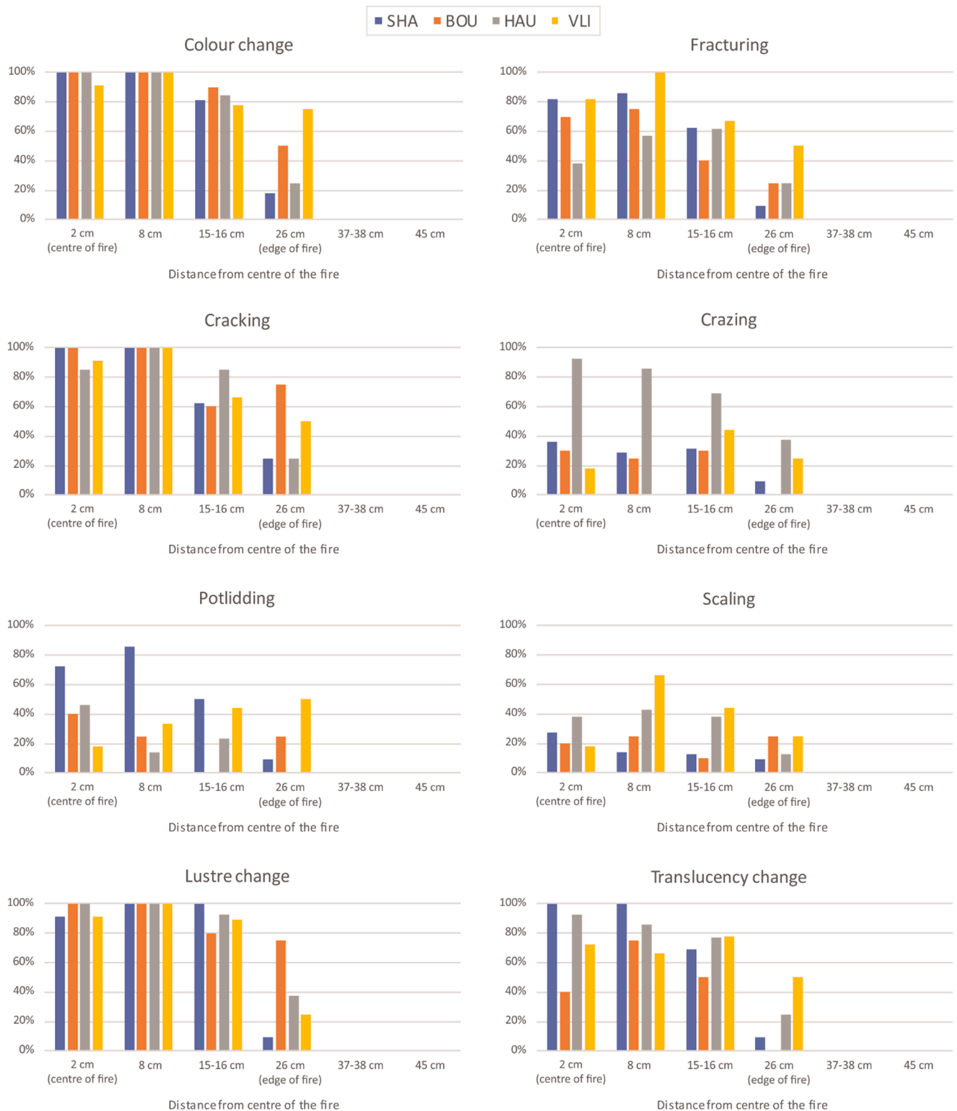
Fig. 11. Connection between position in the fire and appearance of alteration feature by raw materials based on fire 5, 6 and 7. The position correlates to the maximum temperature, i.e. highest temperatures were measured in the middle of the fire and temperatures are decreasing with larger distance from the centre.
