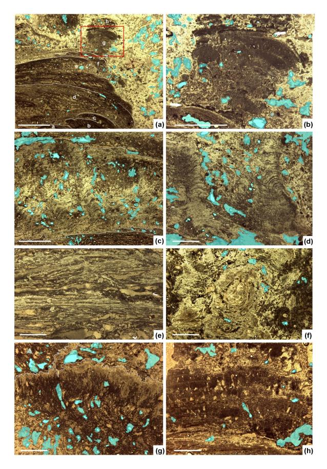
**Figure 4.** Representative optical photomicrographs from the petrographic study of the Seltún sinter exhibiting two-dimensional (2D) textures in transmitted plane light. (a) Superposition of microbial packages (*a* to *h*) showing onlapping features;
