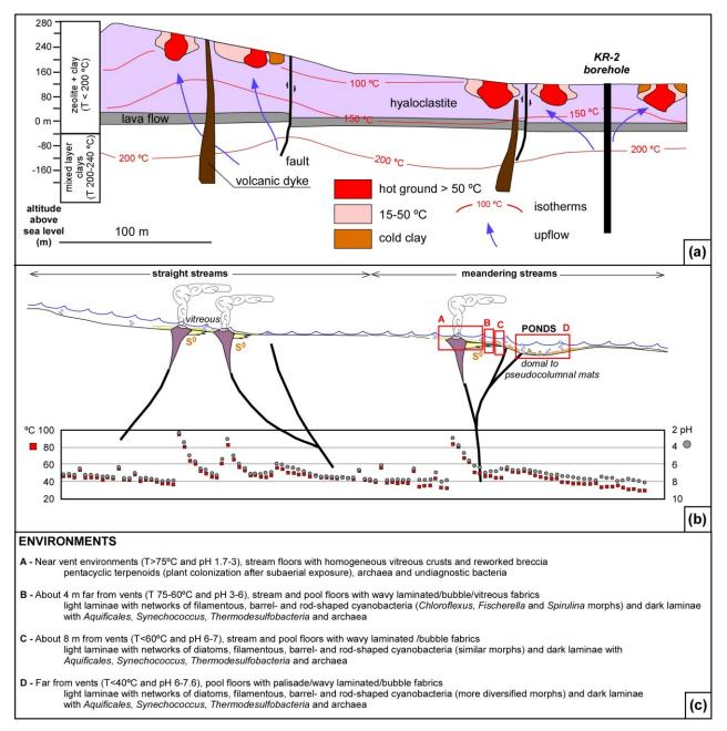
**Figure 11.** Schematic diagram of the Seltún area in the Krýsuvík geothermal. (a) Geothermal model for the Seltún area; modified from [30]. (b) Idealized distribution of fabrics described in the text affected by sharp modifications in temperature and pH conditions of surface waters (measured with a Milwaukee Pro + pH meter; 26 August 2016) controlled by setting of dykes and faults;  $S^0$  abundant native sulfur. (c) Summary of environments and their microbial sinters at Seltún.
