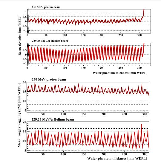
**Figure 9.** Top: The WEPL accuracy of protons and helium for increasing phantom thicknesses. Bottom: The WEPL uncertainty envelope (measured range straggling) of protons and helium for increasing phantom thicknesses, in terms of the width of the  $\pm 2\sigma$  distribution as a metric for layer coverage. The two dashed lines represent the thicknesses of one (8.2 mm WEPL) and two (16.4 mm WEPL) layers.
