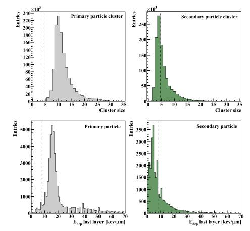
**Figure 2.** Top: The cluster size distribution of primary and secondary hits in the detector prior to track reconstruction. The cut value is  $\leq$  5 pixels per cluster. Bottom: Filter on the  $E_{dep}$  in the last layer, as calculated by the diffused cluster size. The cut value is 8 keV  $\mu$ m<sup>-1</sup>. These figures were made using a 229.25 MeV u<sup>-1</sup> helium beam traversing a 16 cm water phantom.
