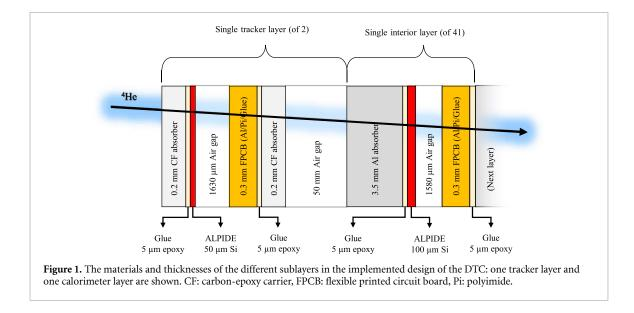
the ALPIDE chip glued onto each side of a 3.5 mm aluminum absorber. A single calorimeter layer has a water-equivalent thickness (WET) of 8.2 mm. The first two layers which form the rear tracker of the device are mounted on two 200  $\mu$ m carbon-epoxy carrier (CF) absorbers for stabilization. This is done in order to reduce the amount of scattering when measuring the position and angle of the particle track, resulting in a layer-wise WET of 1.8 mm.
