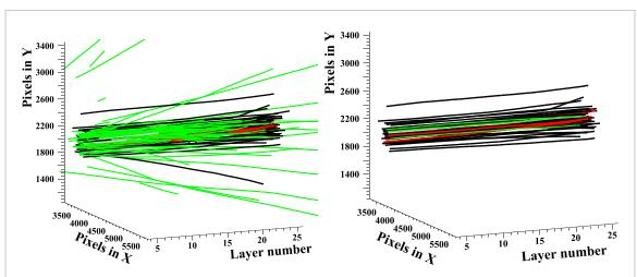
**Figure 7.** A readout containing 100 reconstructed primaries slowed down in 10 cm water. The figures includes 124 tracks before filtering (left) and 45 tracks after filtering (right). A black track is a correctly reconstructed primary; a red track is incorrectly reconstructed due to confusion between two tracks; green tracks are secondaries. Grey tracks are incompletely reconstructed (too short).
