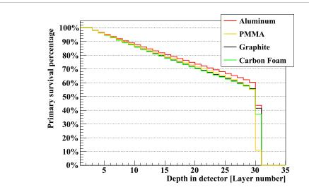
**Figure 6.** The primary helium survival in the DTC for different absorber materials for a 229.25 MeV  $u^{-1}$  helium beam after traversing a 10 cm water phantom. The absorber thickness was scaled to match the WET of 3.5 mm aluminum. The numbers are normalized to per incoming particle.
