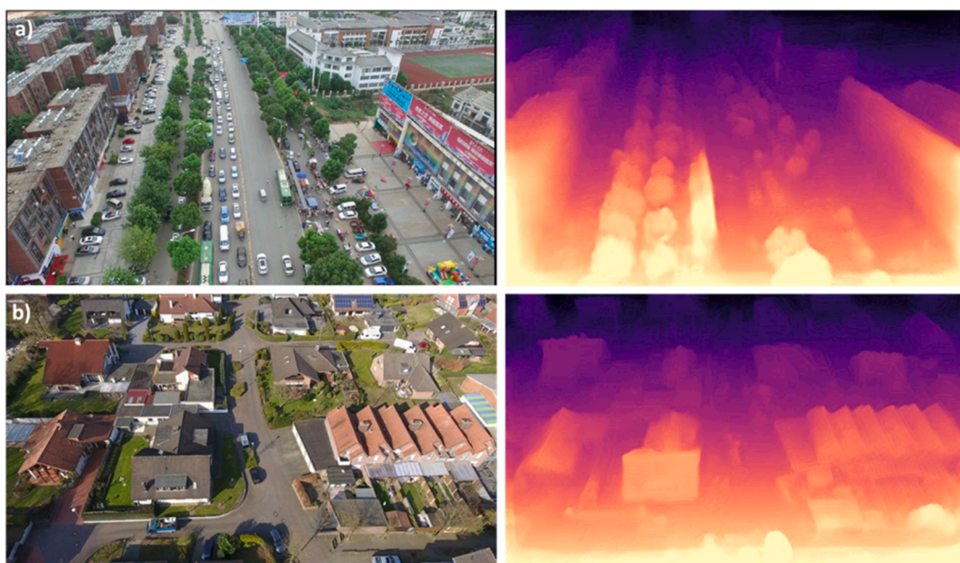
Fig. 1. Disparity from two representative monocular images in UAVid dataset (Lyu et al., 2020) a) Wuhan, China, B) Gronau, Germany.
