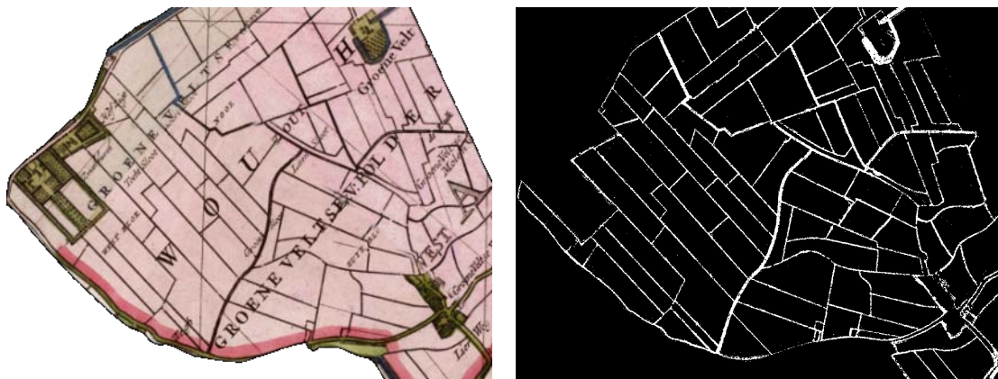
Figure 3. A selection of the original Cruquius map (left) and the derived historic elevation map for the large-scale terrain features added to the generalized historic elevation map (right).
