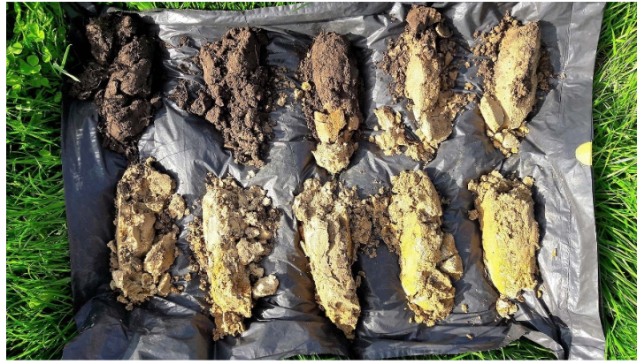
Figure 4. On-site picture of soil sample number 19 (0–100 cm). The topsoil was rich in organic matter followed by a horizon which was brown–red–orange colored due to the presence of iron oxides underlain by a gray–yellow to red–orange sand layer.
