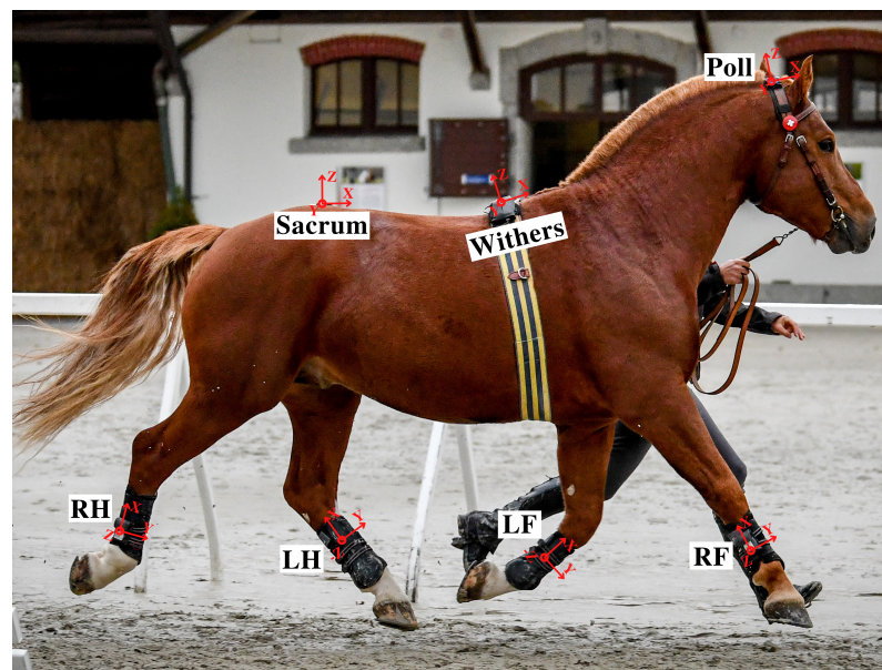
Figure 2. IMUs locations and orientations on horse body. RF: right front limb, LF: left front limb, RH: right hindlimb, LH: left hindlimb. Photographed by Christelle Althaus.
