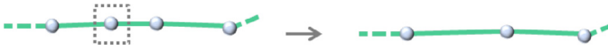
Fig. 7. Illustration of our skeleton pruning process. A skeleton node is removed depending on its associated angle and the lengths of its incident edges.
