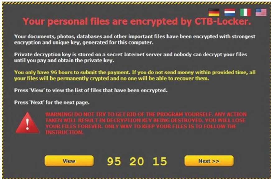
FIGURE 1 Example of a blocking screen demanding a ransom, after the computer system is infected with ransomware. This example concerns the cryptotware known as CTB Locker.
