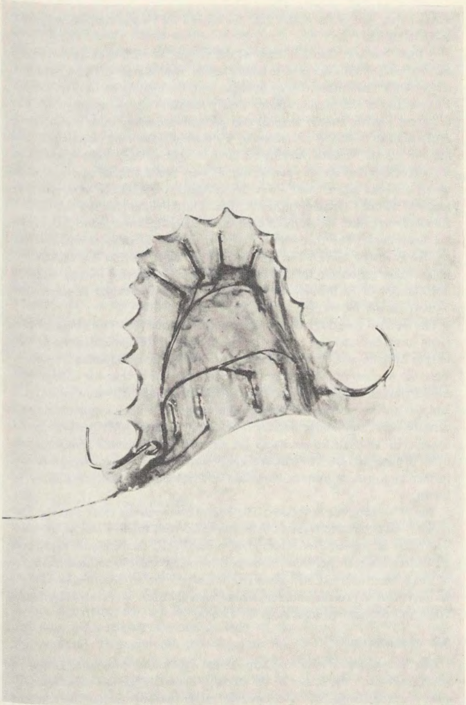
Fig. 2.3. Artificial palate with contacts for measuring tongue-closure durations.
