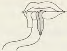
Fig. 2.2. Schematic drawing of the pick-ups used for measuring lip-closure durations.
