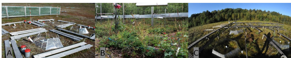
Figure 3.2: In-situ warming experiments: (a) CENPERM OTC set-up on Disko Island, Greenland (b) open-air warming experiment in Kevo, Finland (c) CLIMPEAT OTC in Linje Mire, Poland.
