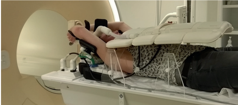
FIGURE 1. Supine patient set-up for MRI simulation. In this set-up a 5 degrees inclined wedges is used. Height-adjustable coil bridges are used as support for the anterior receiver coil to prevent deformation of the body contour.
