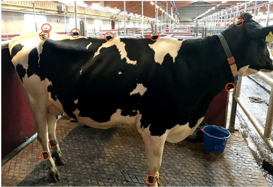
Figure 1. Cow equipped with IMU sensors on predefined anatomical landmarks. IMUs are indicated with orange circles; just caudal to the nuchal crest, the highest point of the withers, the spinal process of the 13 th thoracic vertebra, between the tubera sacrale of the pelvis, right and left tuber coxae, lateral aspect of the metatarsus/metacarpus of each limb and one sensor was attached on the inner right side of neck collar.
