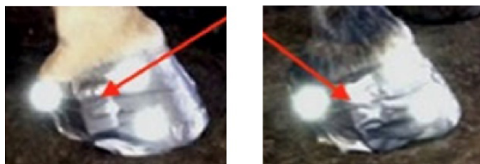
Figure 2. Location of inertial measurement units (IMUs) on the hoof. The location of the IMUs is indicated with red arrows, on the lateral quarter of the right front and hind hoof with reflective markers on both sides (lateral heel, lateral toe and lateral coronet) used for another study (13).
