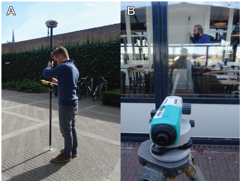
Fig. 3.13. Measurement steps 1 and 3 of the geographical survey. A) Identifying a location with good satellite reception in Culemborg. Photograph by Maarten Zeylmans. B) Difficult levelling measurement of a flood mark in Nijmegen.
