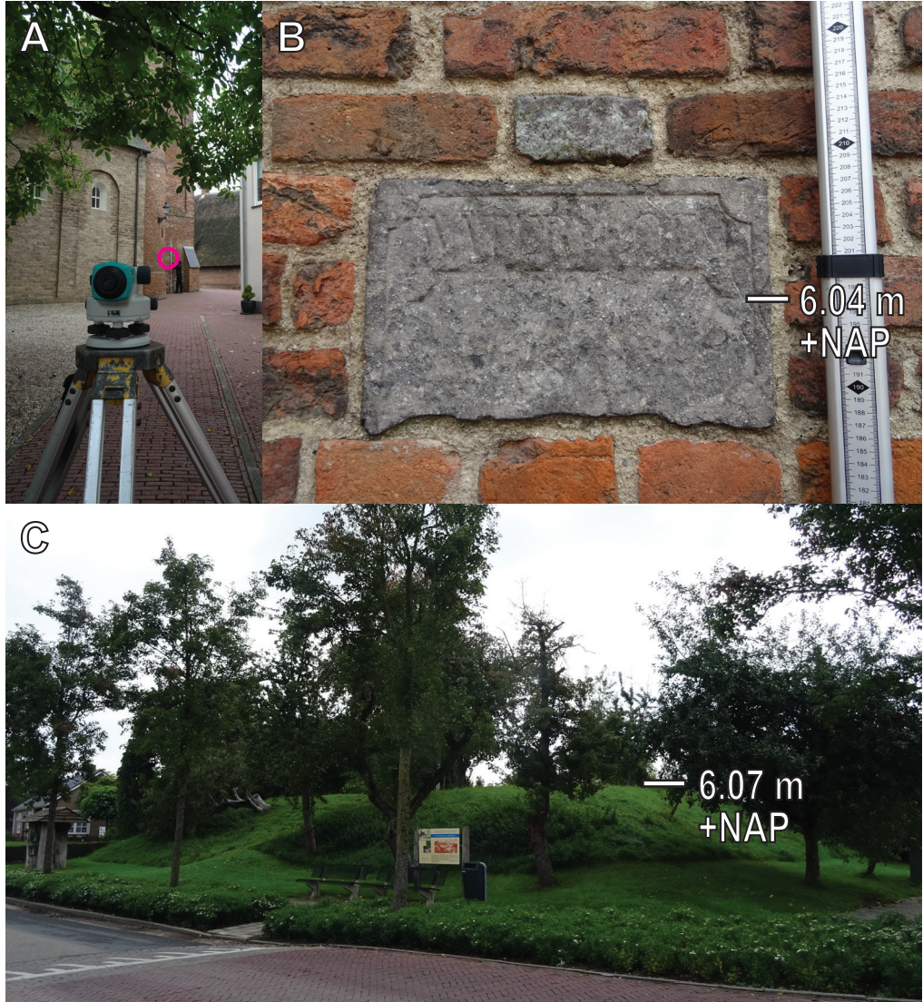
Fig. 3.14. Example of a heavily weathered flood mark in Kerkwijk. A) Position of mark on church. B) Close-up of mark. The nearly erased inscription reads 'WATERVLOED – 1861'. C) Artificial refuge hill located opposite of the church, created as a reaction to the flood. GPS ground level measurements on top of the hill reveal that it was raised to almost exactly the local flood level as indicated by the mark.
