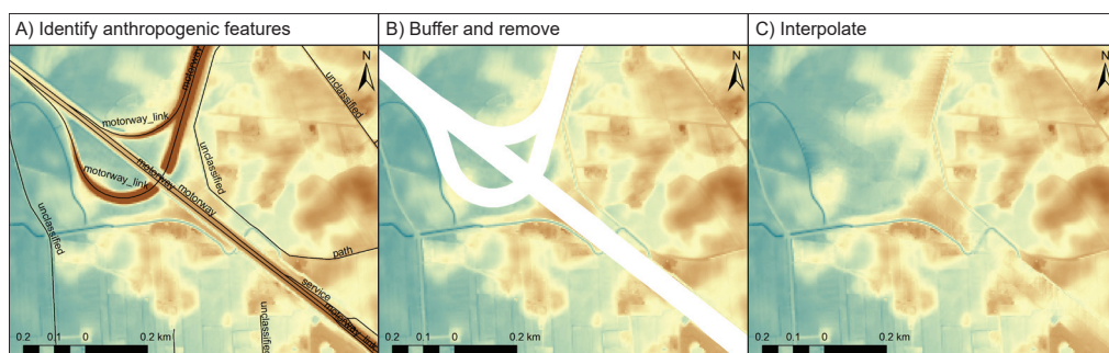
Fig. 5.5. Automated removal of highway-related elevated grounds from the LiDAR ground level DEM. Panel A shows infrastructure vector lines from OpenStreetMap. Panel B shows the applied buffers (widths specified in Table 5.2; see main text for details). Panel C shows the result. Location indicated in Fig. 5.2.
