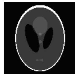
(d) Reconstruction with prior information for the full range setup, but with only a few angles.
