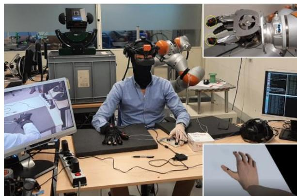
**Figure 1.** Experimental setup (mediated condition). *Top right:* Robotic hand used in the robot condition. *Bottom right:* Human-looking virtual hand in the VR condition.
