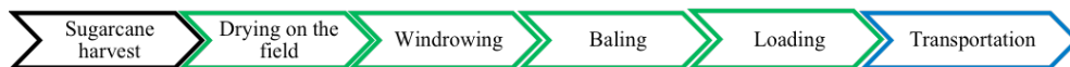
Figure 3.2: The sugarcane straw baling system, including straw operations (in green) and transportation (in blue).
