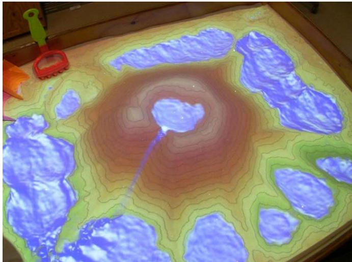
**Figure 3-** AR-Sandbox showing contour lines and water. Colours are projected based on the elevation of the slope (Reed et al., 2016).
