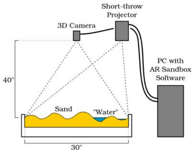
**Figure 2-** The arrangement of projector and sensor to project colours over sand. Retrieved from UC Davis' manual for construction of AR sandbox, <https://arsandbox.ucdavis.edu/instructions/hardware-2/>
