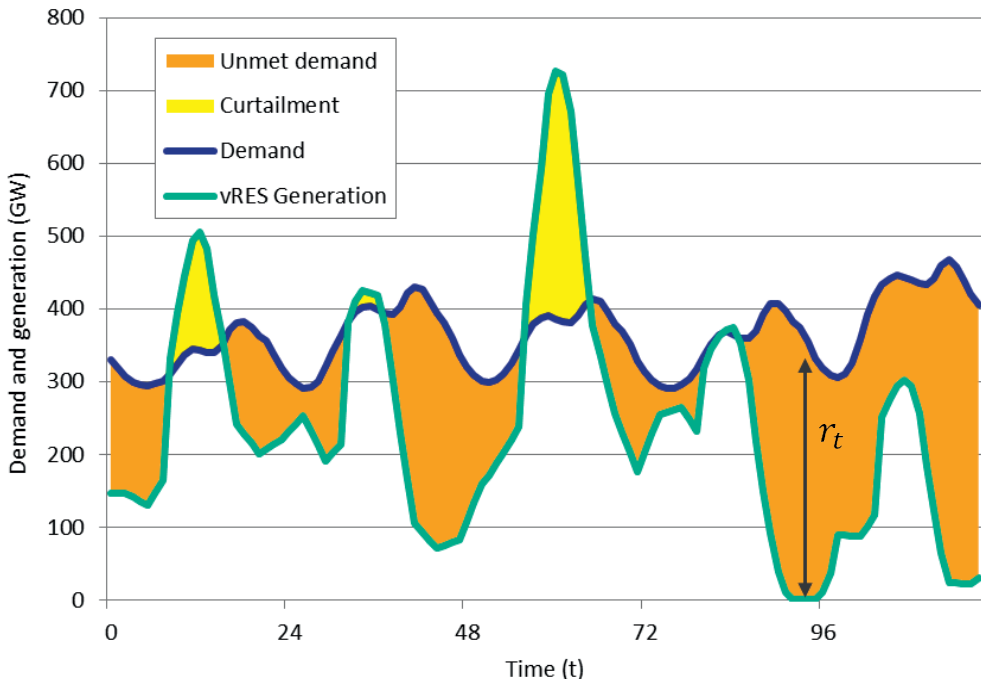
Figure 2-2 | Example of curtailment and residual demand in a power system.
