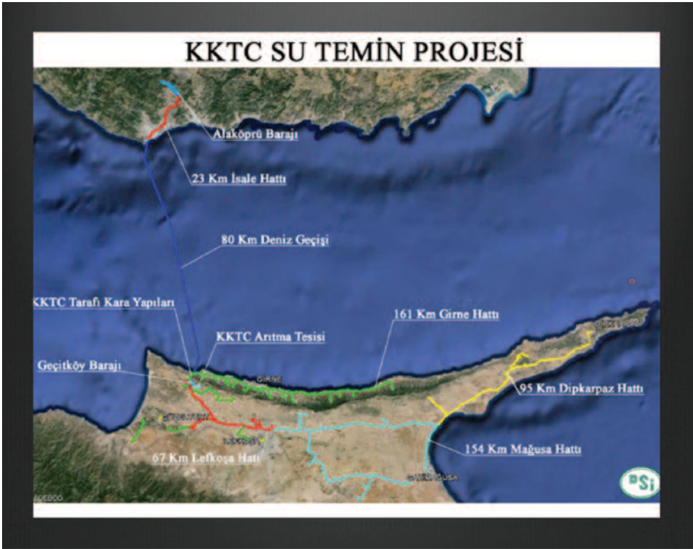
Image 4: Map of the water delivery project from the website of the Turkish Waterworks Department (DSİ), http://www.DSİ.gov.tr/projeler/kkct-su-temin-projesi . The drawing shows both the 80-km undersea pipeline and the distribution network in north Cyprus.
