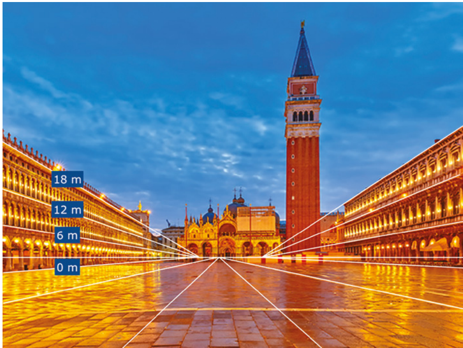
Figure 2. View on of an empty and wet Piazza San Marco. The picture is taken in front of Ala Napoleonica close to positions used by Canaletto. White lines indicate perspective lines converging in the three vanishing points. Indicated heights on the buildings of Procuratie Vecchie have been used as reference for sizes of the central arch of the Basilica (24 m) and the Campanile (99 m) in Canaletto's paintings.
