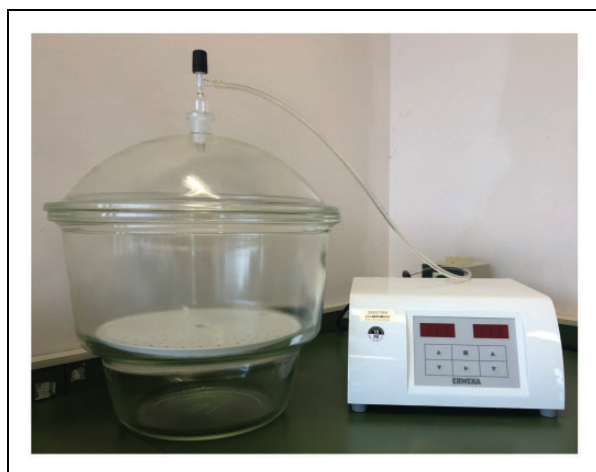
Figure 3. Picture of VDT/S vacuum leak tester with a 300-mm diameter container (Erweka GmbH, Heusenstamm, Germany).
