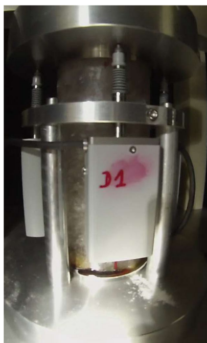
Fig. 11 Hydrocarbons at the bottom of the Go #1 sample device D (left), and displacements during Stages 1 and 2 (right). The four vertical displacements ( D1 - D4 ) are shown together with the averages
