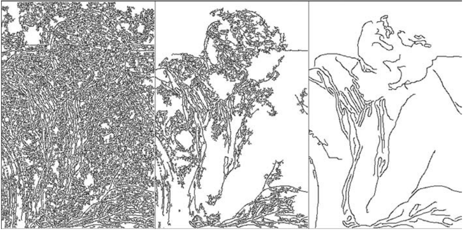
Figure 23. Left: Here I ran the ‘Canny edge detector’ on part of the Boucher painting (Fig. 6, right). Centre: Here I increased the threshold by a factor of three in order to skip ‘weak edges’ (there is an edge — often ‘weak’ — at any pixel for zero threshold!). Right: Here I increased the scale from one pixel to four (threshold the same as in the left-hand picture). You don’t ‘find’ edges as much as you define them by tweaking parameters.
