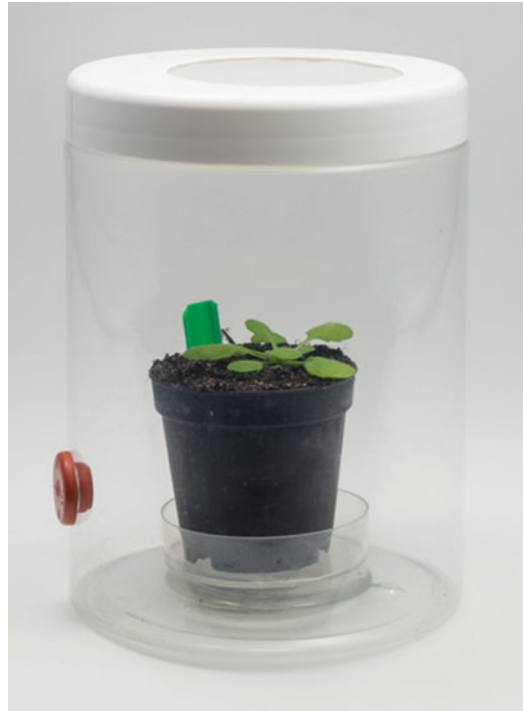
Fig. 2 Modified PET-container for thrips larval rearing and whole-plant bioassays
