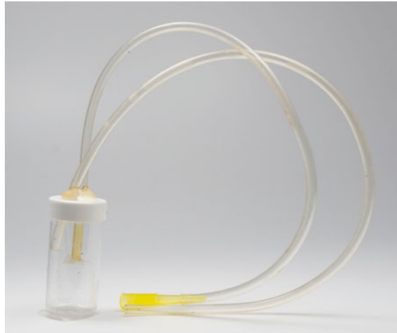
Fig. 4 Handmade aspirator to collect thrips
