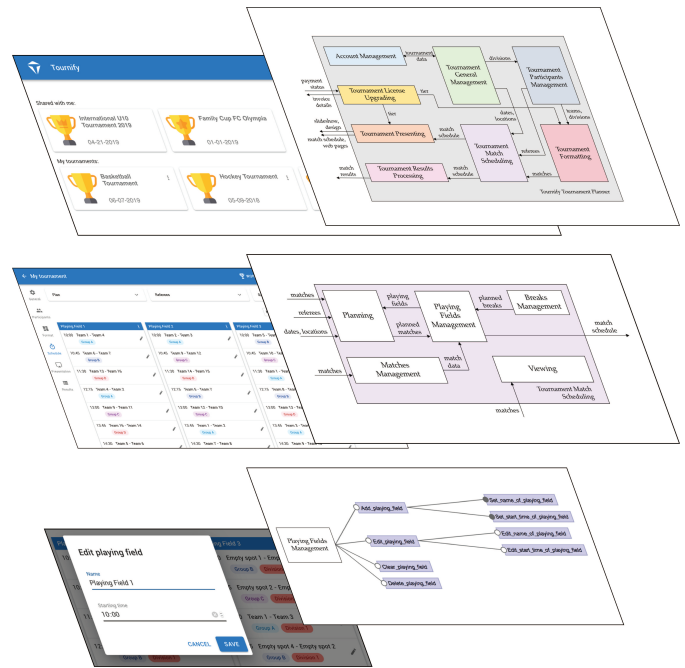
Fig. 5. Three-layered functional architecture of a web application, recovered based on the GUI.
