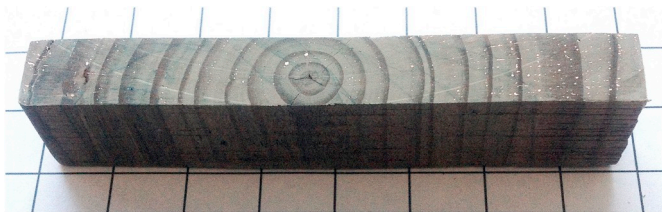
Fig. 3. Slice of pit prop sample studied. Note fine light-colored grains of native copper. Approximate size of sample 7.5 cm long, 1 cm wide, and about 2 cm high.
