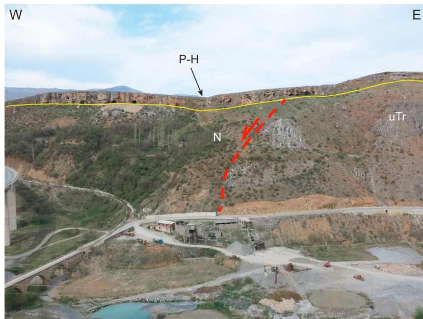
Figure 6. Miocene normal faulting at northern side of the entrance to the Luma Gorge near Kukës, NE Albania. Normal fault (red dashes with motion arrow of hanging wall) juxtaposes Upper Triassic limestone (uTr) of the Korab-Pelagonian Nappe in the footwall with Pliocene conglomerates (N) in the hanging wall. This faulted sequence is overlain by Pleistocene-Holocene terraces (P-H, above yellow line), which are in turn faulted and warped into a gentle monocline. Photo location coordinates: 42° 3'58.20"N, 20°27'54.39"E.
