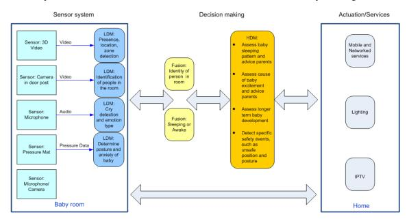
Figure 1. High level infant monitoring architecture consisting of three stages: sensing, reasoning and actuation.
