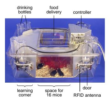
Figure 1. The IntelliCage apparatus.
