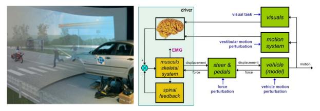
Figure 1. Driving Simulator; a human operator interacts with a virtual vehicle in a virtual driving environment. The driver receives visual task stimuli and various perturbations and driver actions and vehicle responses are recorded.
