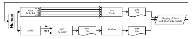
Figure 1. An overarching framework or processing pipeline for mapping the Xsens body suit data and the Kinect data upon each other.
