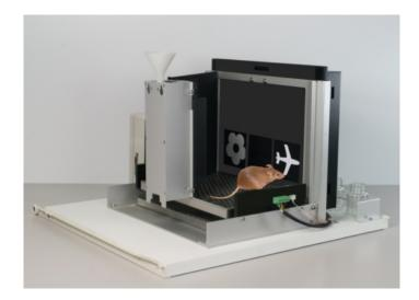
Figure 1. Touchscreen testing setup.
