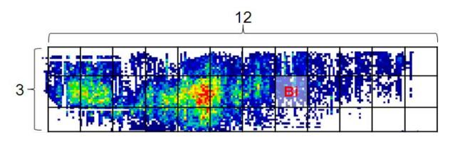
Figure 2. Pressure frame of left-side posture with the head on the left and the legs on the right. A grid of 3x12 is applied by summing the pressure in each cell.
