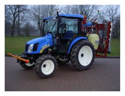
Figure 1. Autonomous tractor used to apply pesticides in strawberry fields. At present, the only safety feature of this tractor is the front-mounted bar with emergency stop buttons at either end.
