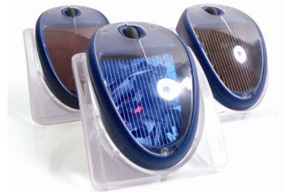
Figure 1: Photographs of three Sole Mio prototypes, each equipped with a different solar cell type.
