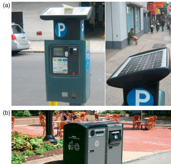
Figure 6 Examples of PIPV business-to-business products. (a) Parking meter in New York City. (b) Automated trash bin Big Belly.
