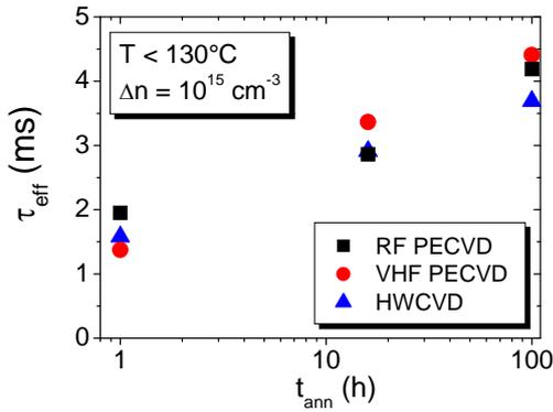
Figure 1, Minority carrier lifetimes at an injection level of  $10^{15} \text{ cm}^{-3}$  plotted against anneal time for the three different deposition methods.
