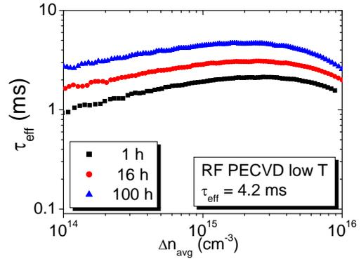
Figure 2, Injection level dependent minority carrier lifetimes of the sample deposited by RF PECVD after 1 h, 16 h and 100 h of thermal annealing at  $200^\circ\text{C}$  in  $\text{N}_2$ .
