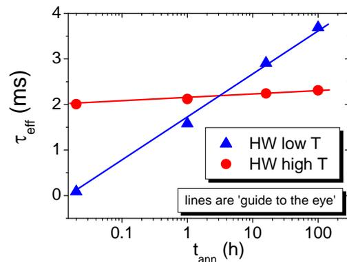
Figure 4, Annealing characteristics for low T (120°C) and high T (250°C) passivation samples made by HWCVD. The lines are a guide to the eye.
