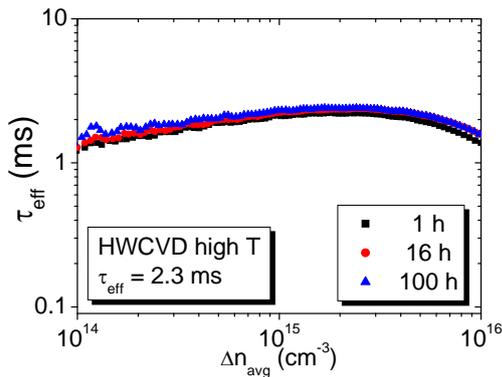
Figure 3, Injection level dependent minority carrier lifetime of a HWCVD sample deposited at 250°C after 1h, 16 h and 100 h of annealing in N<sub>2</sub>.
