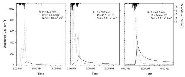
**Fig. 4** Hydrographs observed in the former agricultural (dotted line) and forested (solid line) catchments for different preceding conditions. P: rainfall depth; IP: mean rainfall intensity; Qini: baseflow discharge at the start of the event.
