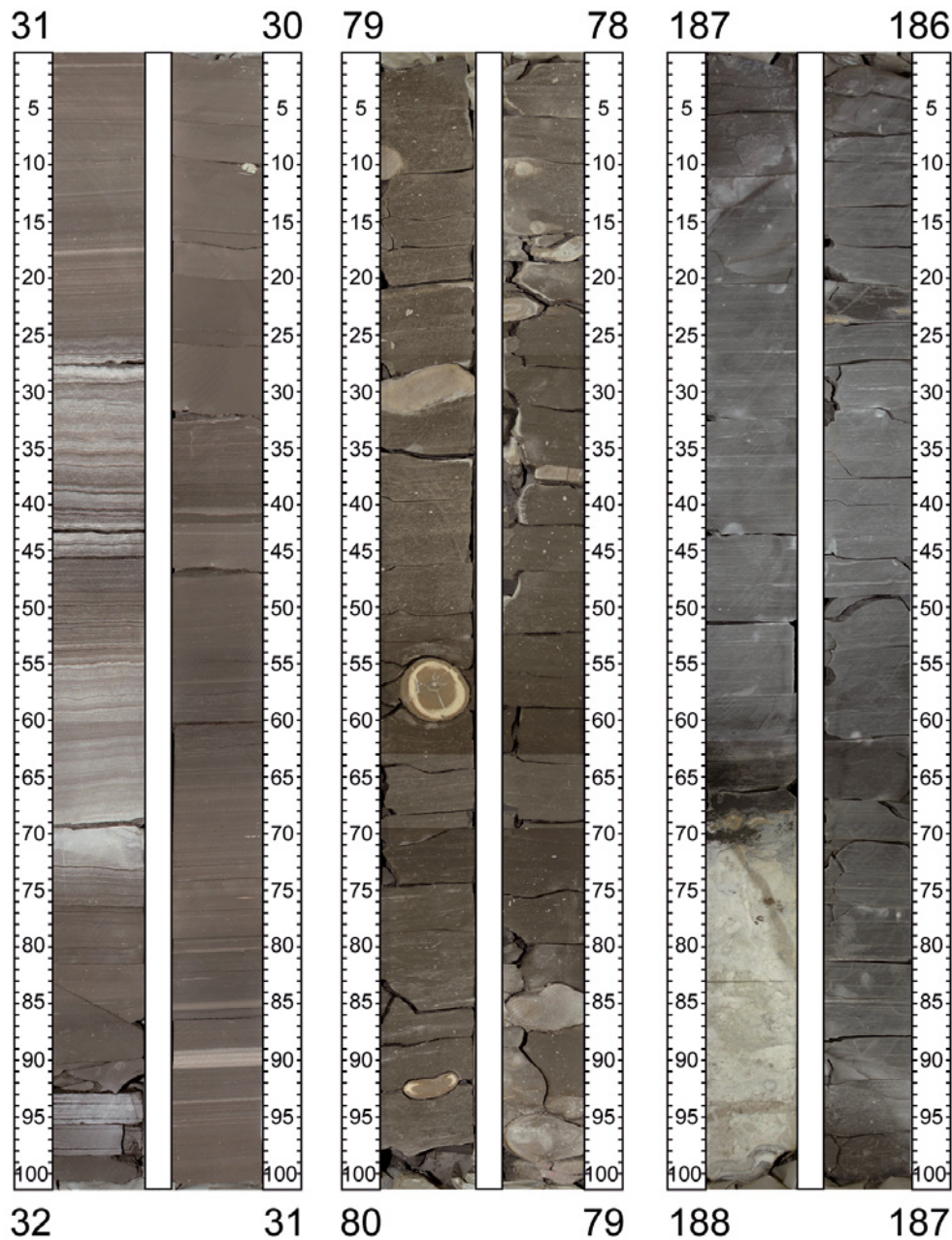
Plate 9. Examples of typical lithological features of the Toarcian, Pliensbachian and Sinemurian (from left to right). Core section 30.00–32.00 mbs: Example of laminated paper shales of Toarcian age. Within this section of the Toarcian, several calcareous beds can be recognized that have wavy laminations. The unique nature of these beds suggest that these represent the so-called “Monotis Bed” that marks the base of the Bifrons Zone. Core section 78.00–80.00 mbs: Lithofacies of the Upper Pliensbachian Margaritatus Zone. This part of the Pliensbachian is very rich in carbonate concretions with complex diagenetic histories. A zoned septarian nodule is present at 79.55 mbs, which is likely sideritic. Other more tabular concretions occur dispersed throughout this core section. Core section 186.00–188.00 mbs: Example of lithological variations in the Sinemurian. A 30 cm thick hardground bed containing lithoclasts occurs at 187.70 mbs and was identified as the Upper Sinemurian “Konglomerat-bank” (Oxynotum Zone).
