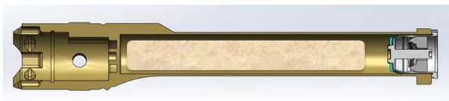
Fig. A3.1. A returnable Mars 2020 sample tube assembly with a schematic illustration of a collected core. On the left is the interface with the drill, on the right is the open end of the tube, which is shown in this drawing after the hermetic seal has been installed. The rock sample (tan color) is shown schematically, but we expect almost all samples to be fractured, and in some cases, heavily so. Total length of the tube is ~15 cm. The sample cavity is ~13.2 mm × 100 mm, while the inner diameter (ID) of the cutting bit is 13 mm, resulting in an average size of collected cores of slightly less than 13 mm diameter. In tests on a range of analog materials the average size of collected cores was ~13 mm in diameter × 60 mm in length.
