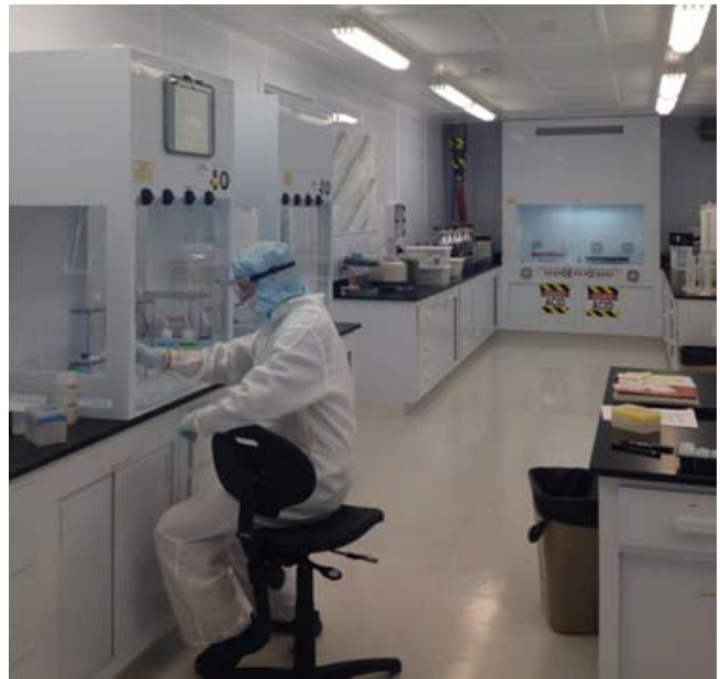
Fig. 3.3. For state-of-the-art high-precision radioisotope analyses, sample handling and chemical processing in a clean laboratory such as the one shown here are typically required. Image credit: Center for Meteorite Studies at Arizona State University.
