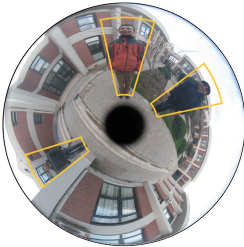
Fig. 1 Person detection in an omnidirectional camera setting, with the detection results of the proposed approach superimposed
