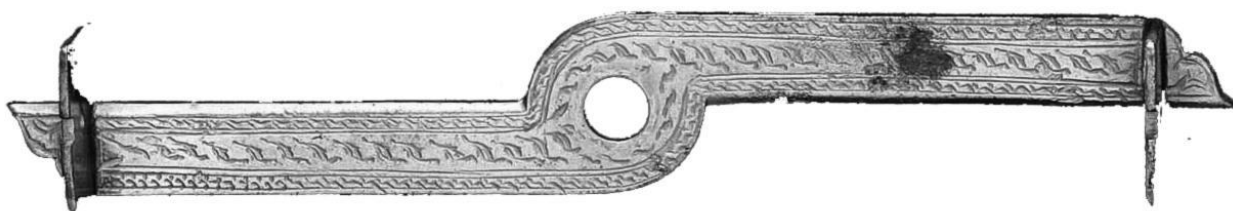
Figure 1-1b: Counterchanged alidade, made in the late 9 th century A.D., Syria; Oxford Astrolabe Collection, above: no. 47632 ( https://www.mhs.ox.ac.uk/astrolabe/ ) [CCA 1026]
