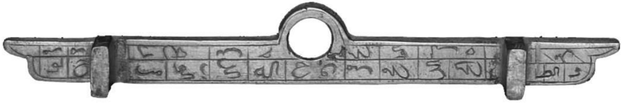
Figure 1-1c: Straight-bar alidade, made in the early 18 th century A.D., Iran; Oxford Astrolabe Collection, no. 37940 ( https://www.mhs.ox.ac.uk/astrolabe/ ) [CAA 1021]
