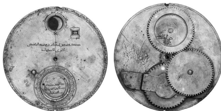
Figure 0-5. The front (left) and back (right) of the lunar-box. This device indicates the number of the day in the lunar calendar as well as the corresponding phase of the moon, and the position of the moon and the sun. Made in 1221-2 A.D., Isfahan, Iran; Oxford Astrolabe Collection, no. 48213 [CCA 5]
