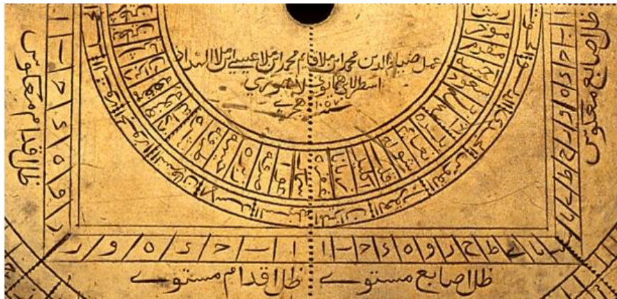
Figure 3-4. The ladder shadow ( zill al-sullam ) with two squares on the back of the astrolabe, made in the 17 th century A.D., Lahore, Pakistan; Adler Planetarium Collections, no. A-70 ( http://www.adlerplanetarium.org/collections/ ) [CCA 1095] The semicircle contains astrological information which is of no concern to us.
